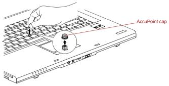
Figure 4-2 Removing the AccuPoint cap
